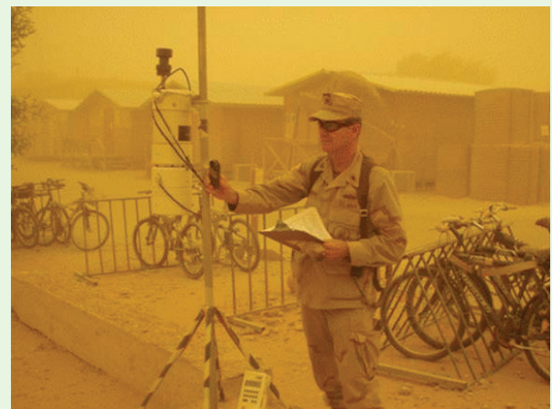
Figure 3-1. The author using the MiniVol Portable Air Sampler (Airmetrics, Eugene, OR) during a 2008 dust storm in Al Asad, Iraq.
